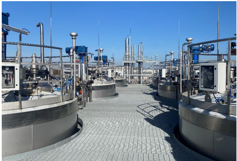
All the large-scale fermenter vessels are now fully commissioned and operational, pictured with the distillation columns in the background.
